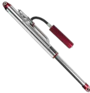
A combination of the 2.5 Remote Reservoir Triple Bypass Shocks and the Profender 4x4 Air Shocks, giving the best of both worlds
