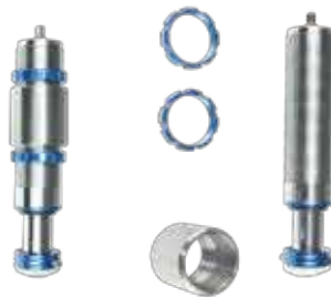
Adjustable Bumpstops in 2.0 with 2" & 3" travel. Up to 170mm in height adjustment.
