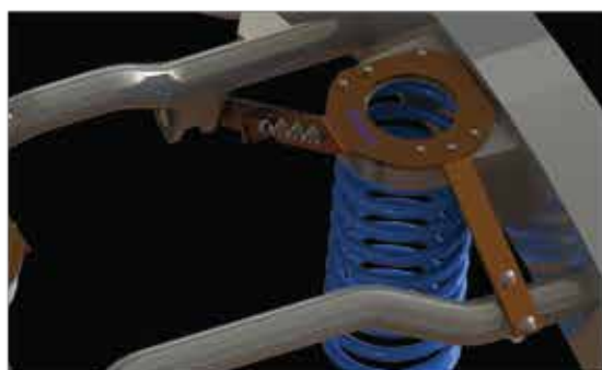
CAD(computer aided design) used to ensure a perfect fit within the minimal space available.
